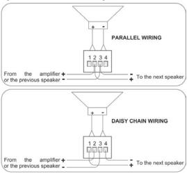
Figure 3: SPK-C612 Schematic Diagram
